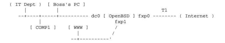
In this example, the OpenBSD host is acting as a firewall for a company network. The company runs a WWW server in the DMZ portion of their network where customers upload their websites via FTP. The IT department has their own subnet connected to the main network, and the boss has a PC on his desk that's used for email and surfing the web. The connection to the Internet is via a T1 line running at 1.5Mbps in both directions. All other network segments are using Fast Ethernet (100Mbps).
